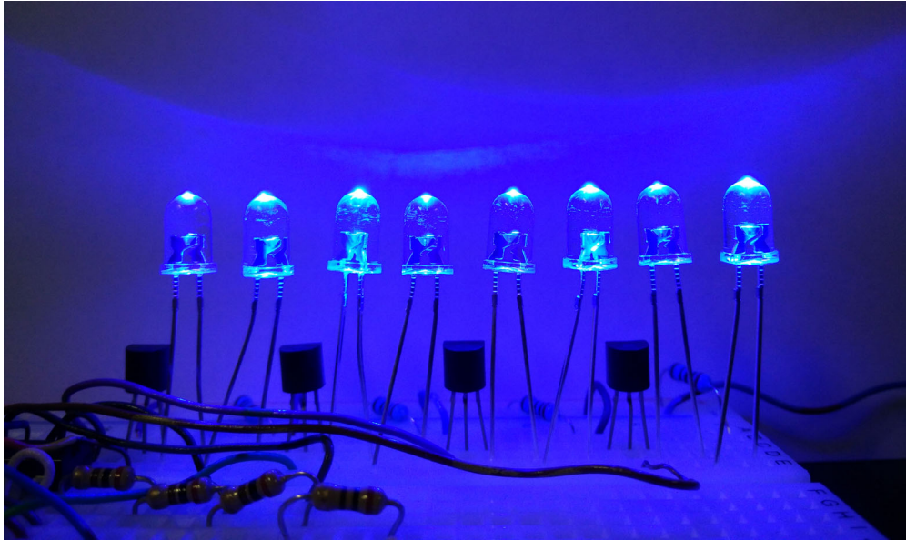
Figure 29: All the lights are turned on when the amplitude of the noise saturates the voltage seen across the series of resistors
